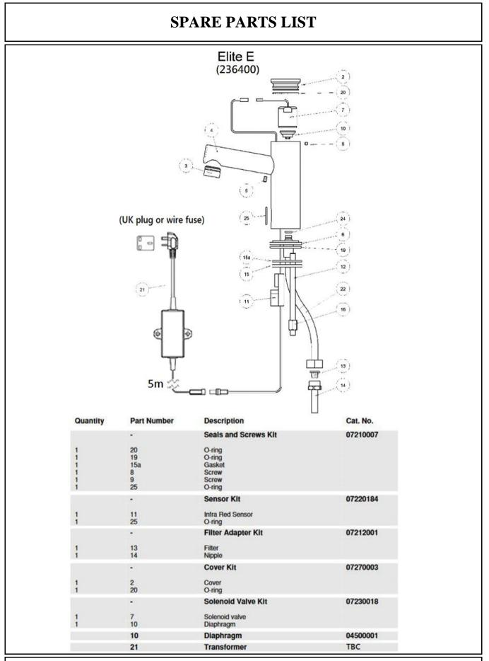
Note: In order to locate the relevant spare part, please check the corresponding parts and part mumber in the drawing. Minimum order quantity will be required.
